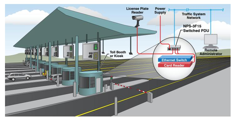
In Toll Booth applications, the NPS-3F15 Network Power Switch is often used to provide a means to remotely reboot devices such as card scanners, tag readers, toll collection systems, license plate capture cameras and other networked devices. When any of these devices fail, remote administrators can immediately establish a secure connection to the NPS unit and then initiate power reboot operations to restart nonresponsive devices and restore normal operation.
