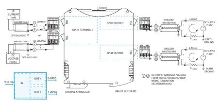
DC current and low voltage input ◆ 4-20mA outputs (sink/source) ◆ 7-32V DC loop power
