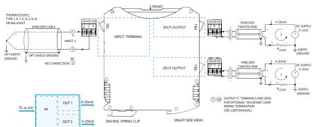
Universal thermocouple or ±100mV input ◆ 4-20mA outputs (sink/source) ◆ 7-32V DC loop/local power
